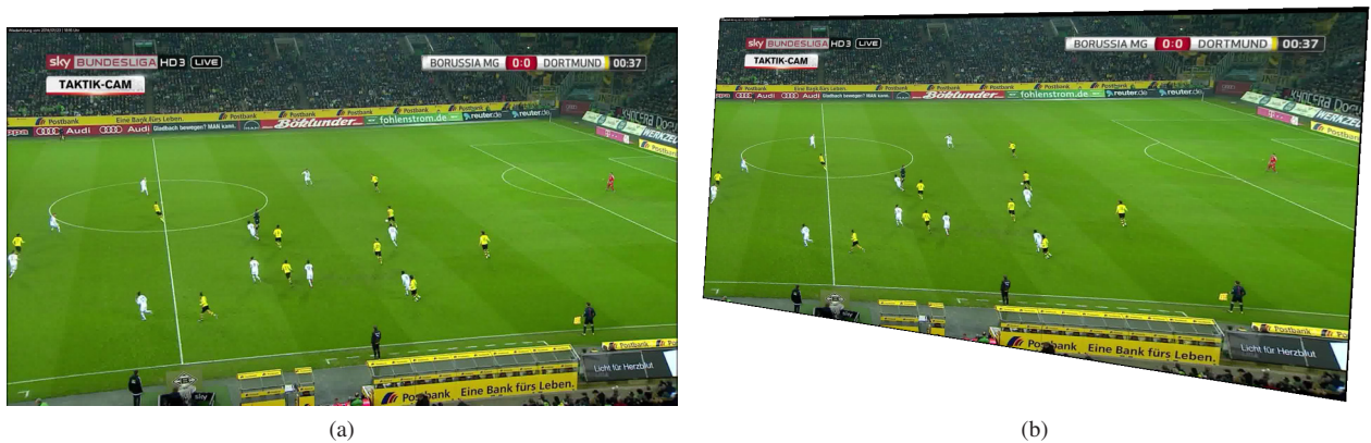
Fig. 5: Before homography (a) and after homography (b) calculation.
