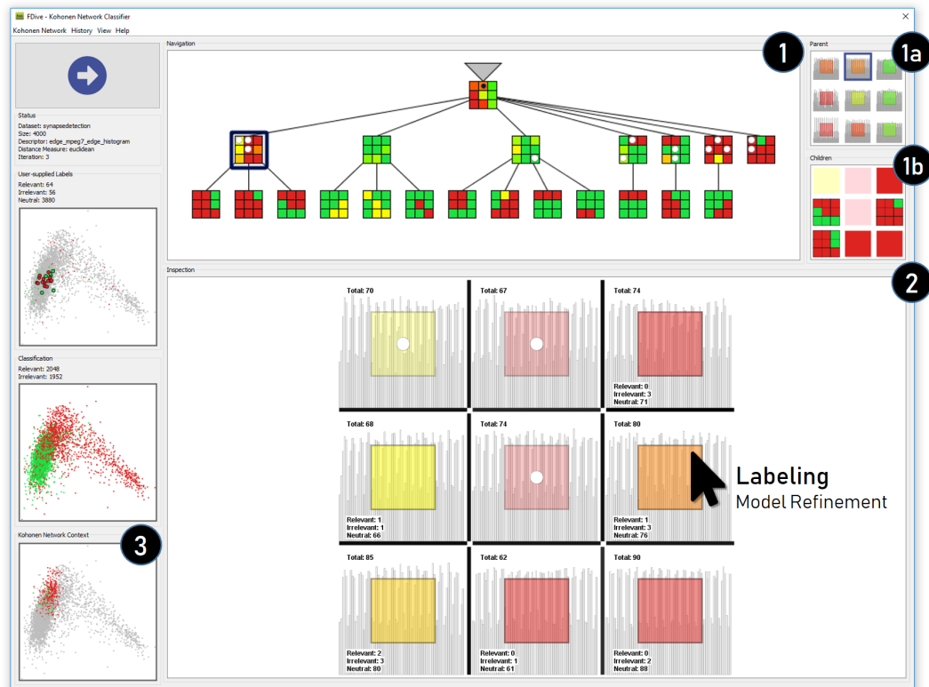
Figure 6.5: Visual Exploration of SOM Model: 1) Classifier tree. 1a) Parent of the currently observed SOM. 1b) Children of the current SOM. 2) Detailed SOM Display. 3) Scatter plot highlighting data of the SOM node.
