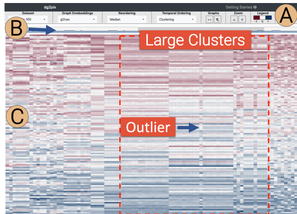
Figure 3: The dg2pix component consists of three views a toolbar (A), the zoom context bar (B), and the pixel-based visualization (C). In (C) the embeddings (GL2Vec [14]) of a synthetic dynamic graph (SBM [25]) with reoccurring states are depicted. The displayed embeddings of the x-axis are clustered (HDBSCAN [13]), and y-axis ordering is based on the median of each vector attribute. The reordering and clustering of the synthetically created reoccurring states highlight large clusters of similar graphs and outliers in the temporal data.
