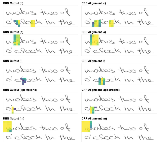
Figure 6: Heat maps of top-5 characters when using Difference as the sort criterion. Difference sort criterion is useful for quickly spotting the characters with the largest disparity between the network output and alignment. It is thus suitable for finding general improvements in hyper-parameters. Left column shows the predicted probabilities, right column the alignment probabilities.
